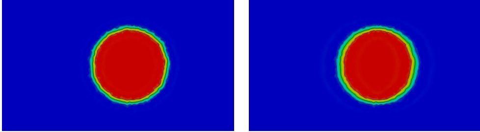
Fig. 14 Zoomed solution and contour lines of 0.1, 0.5, 0.9 for k = 2 with CFL = 0.5 (left) and 10 (right)
